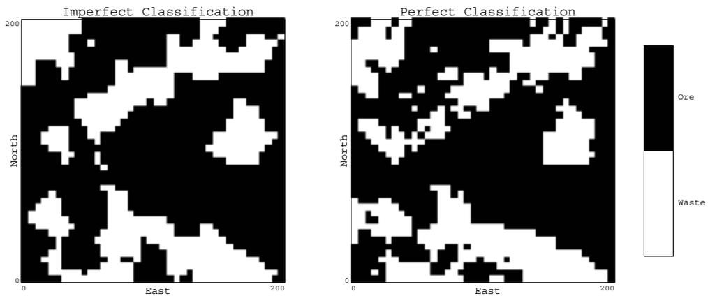
**Figure 6:** Comparison of imperfect and perfect ore/waste classification. The imperfect classification is on the left and the perfect classification is on the right.
