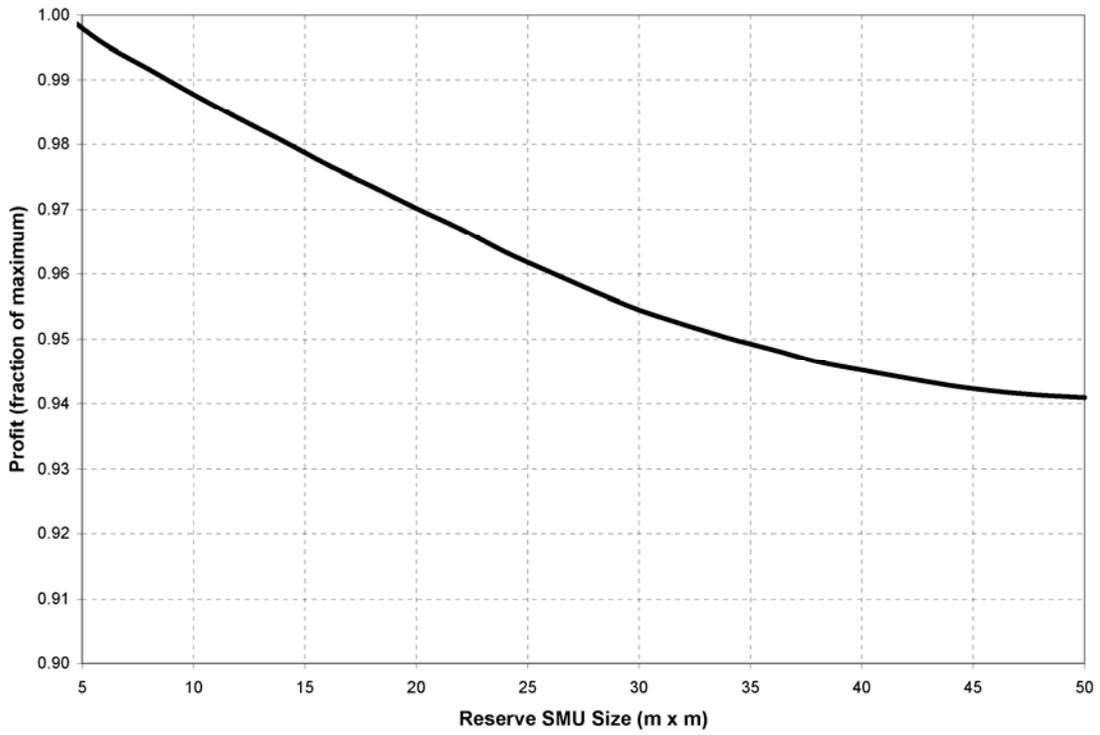
**Figure 4:** Profit from the Discrete Gaussian model versus SMU size.
